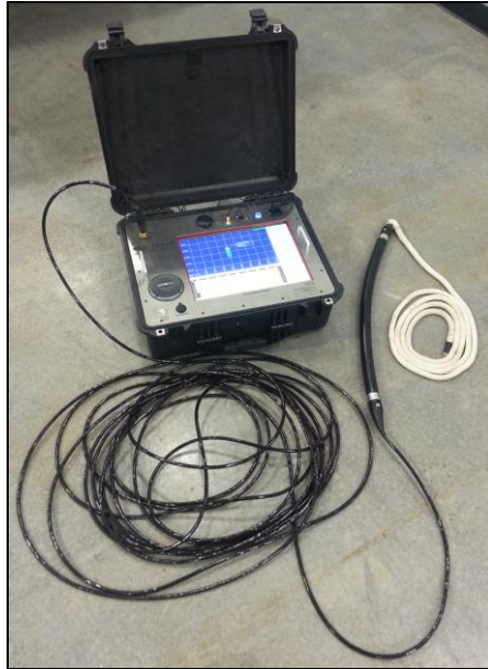
Figure 4 - SeaTrack Deck Box, Towable Hydrophone with Rope Drogue
