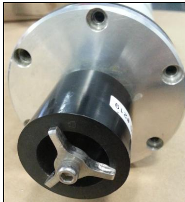
Figure 3 - SeaTrack's Free Flooding Ring (FFR) transducer
