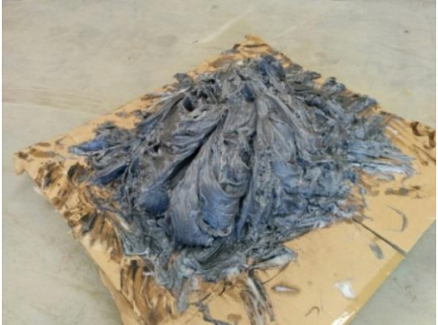
TEST 1: Soft Paraffin wax mixed with black dye
