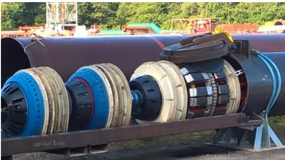
Figure 4: MFL tool during check valve testing
