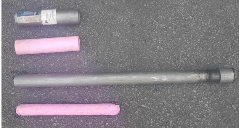
Fig. 7: Full size EVO-Pig and canister and EVO-Pig removed from 2" pipe after few weeks
