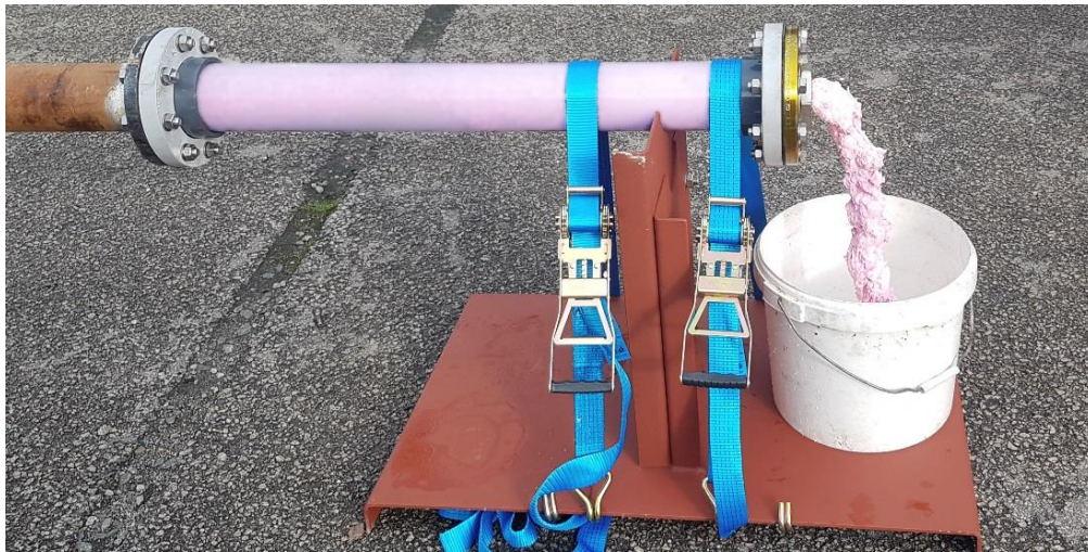
Fig. 1: Extrusion of welding plug using 1.5" port from 4" pipe
