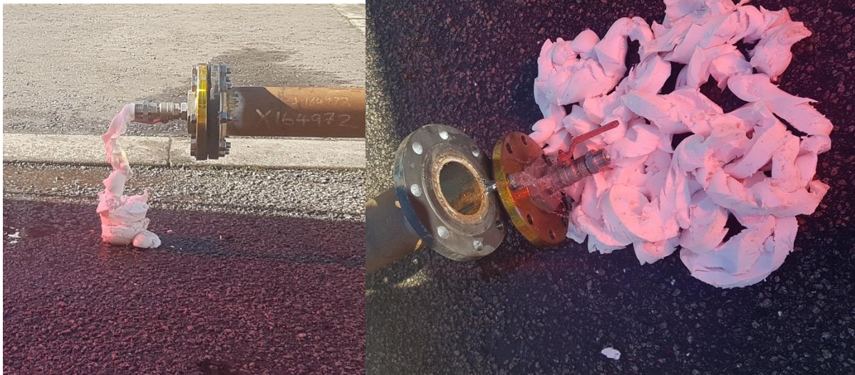
Fig.9: Extrusion of 4" diameter 1230mm long welding pig
