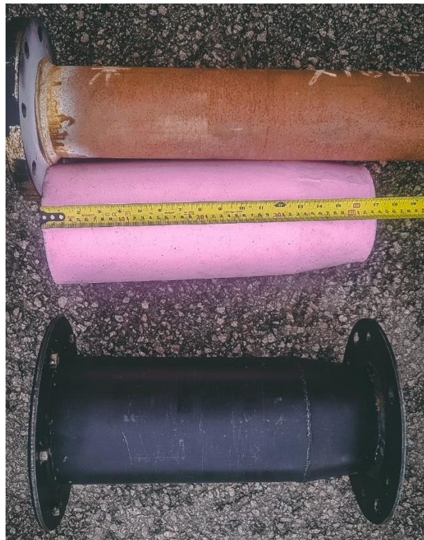
Fig. 8: Fresh EVO-Pig removed from manufacturing canister alongside 4" pipe
