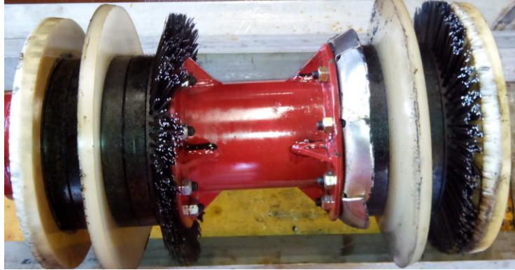
Figure 5: Standard Steel mandrel Gauge pig with added brushes
