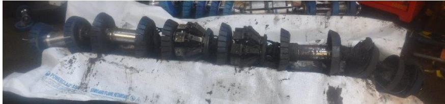
Figure 13: UT Inspection tool after run in 2019
