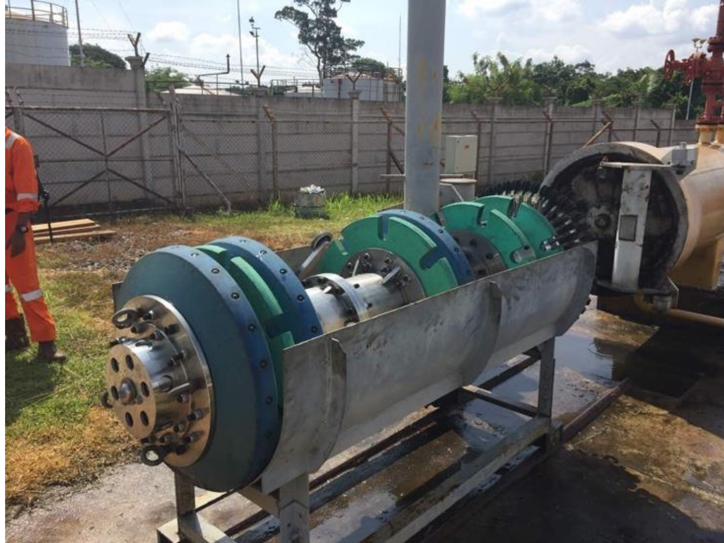
Receiving the 28" High Resolution Geometry + IMU Survey Tool
