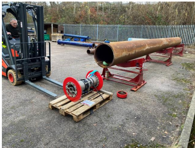
Figure 4: Test pipe with pig ready to be inserted
