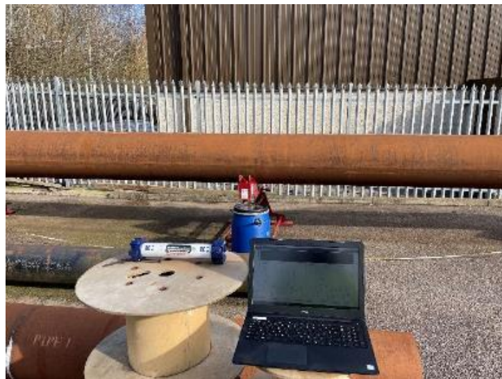
Figure 6: EMRx positioned 1m from pipe centre
